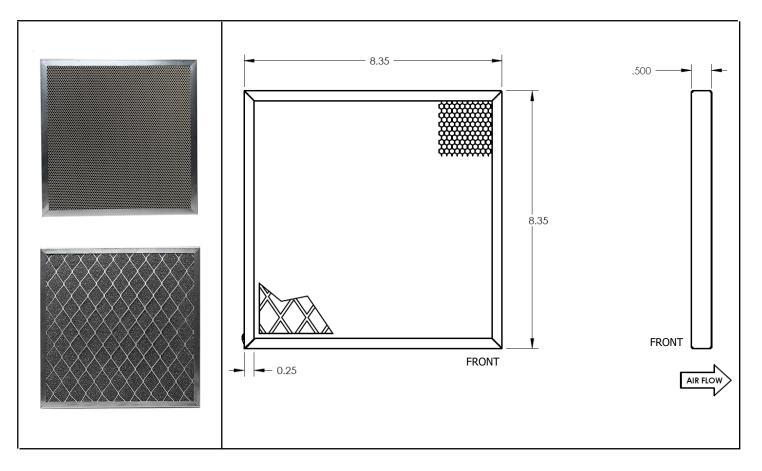
Orion Fans Pyrocide filters meet stringent flame safety standards for fire containment in electronics enclosures by preventing flames from propagating through the vent panels. The pyrocide coating has an ASTM E-84 Class A rating with low flame spread and low smoke index values. A thin coating in the honeycomb cells reacts on exposure to flame and expands rapidly, to prevent flames from propagating through the vent panels.
