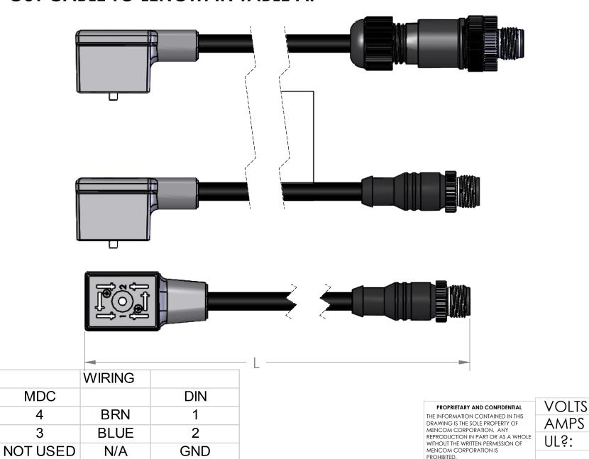
NOTE: CABLE MUST BE CUT TO PROPER LENGTH BEFORE **ADDED CONTACTS TO THE** WIRES.
