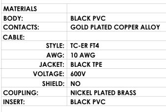
**RATINGS** SCCR RATING: 65 kA Breakers and Fuses YES ROHS COMPLIANT: IEC IP67 PROTECTION: PVVA (US), PVVA7 (Canada) **UL CATEGORY:** U.S.: UL 2237 LISTED, File E469485 CANADA: C-UL 2237 LISTED, File E469485
