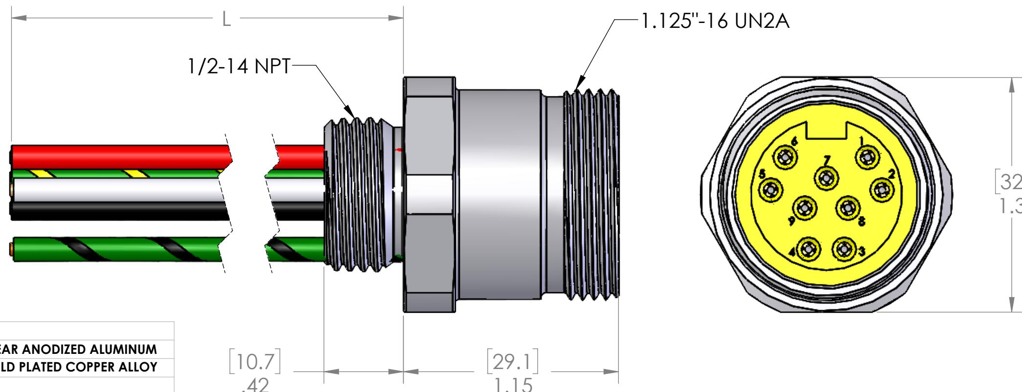
AN O-RING AND LOCKNUT ARE INCLUDED
