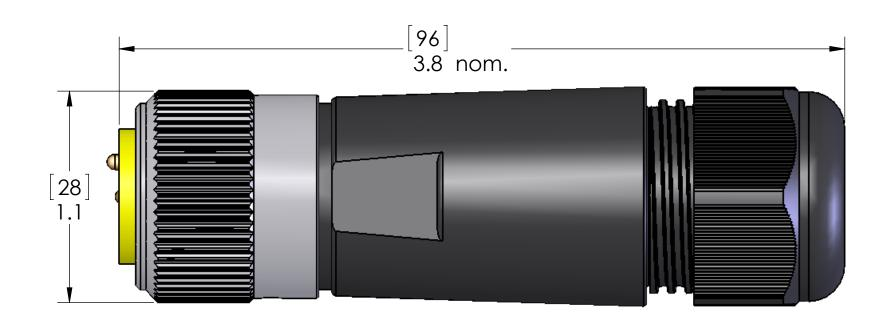
**MATERIALS** BODY: **BLACK POLYAMIDE CONTACTS: GOLD PLATED COPPER ALLOY CABLE SEAL: NBR INSERT:** YELLOW PVC **COUPLING: NICKEL PLATED BRASS RATINGS** 16AWG - 8A max AMPS: 18AWG - 5.5A max 20-22AWG - 4A max **VOLTS:** 600V MAX SEAL: IP67 CABLE RANGE: 16AWG - 22AWG 0.31" - 0.67" (8mm - 17mm) OD **APPROVALS** (16-20AWG ONLY) US: **UL LISTED** CANADA: **C-UL LISTED**
