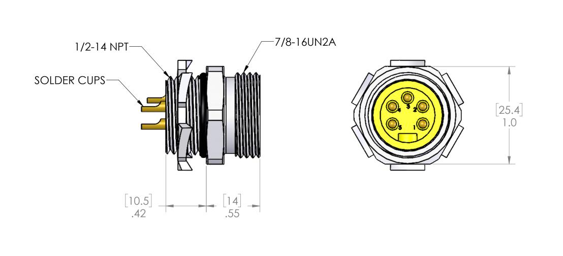
**MATERIALS** SHELL: **CLEAR ANODIZED ALUMINUM** CONTACTS: GOLD PLATED COPPER ALLOY INSERT: YELLOW PVC O-RING: NBR NUT: ZINC PLATED STEEL **APPROVALS** A US: **UL LISTED** C-UL LISTED CANADA: ROHS: YES CE & UKCA: YES RATINGS PROTECTION CLASS: UL TYPE 4 & 12, IEC IP69
