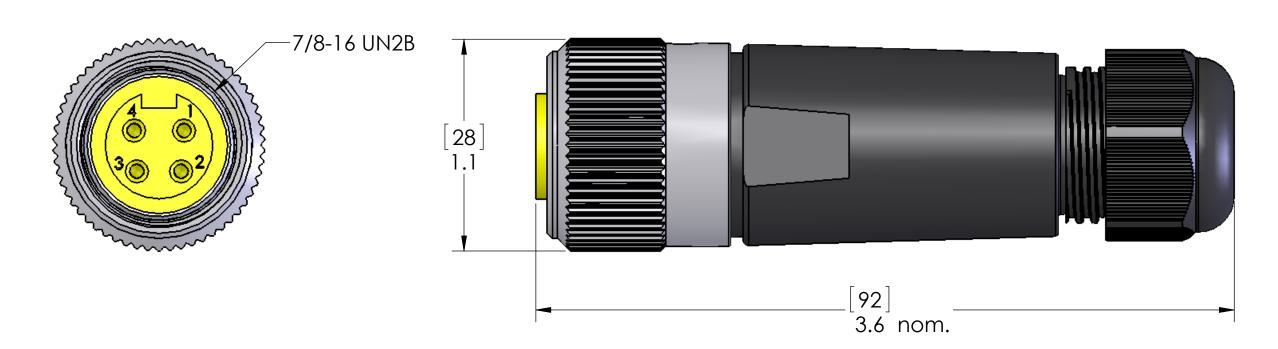
**MATERIALS BLACK POLYAMIDE BODY: GOLD PLATED COPPER ALLOY CONTACTS: CABLE SEAL:** NBR **INSERT: YELLOW PVC NICKEL PLATED BRASS COUPLING: RATINGS** AMPS: 14AWG - 15A max 16AWG - 10A max 18AWG - 8A max 20-22AWG - 4A max **VOLTS: 600V MAX** SEAL: **IP67** CABLE RANGE: 14AWG - 22AWG 0.20" - 0.51" (5mm - 13mm) OD **APPROVALS** US: **UL LISTED** CANADA: **C-UL LISTED**
