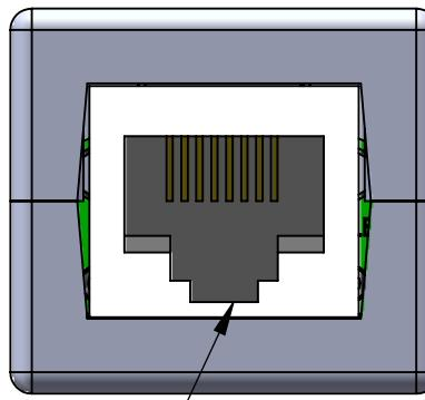
Note: The shield of the RJ45 connector is electrically connected to the shell of the MDE45 Connector. If this connection is not desired, consult factory for the part number for one that is not connected.
