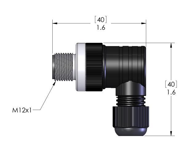
All connections made via Screw Terminals. Keyway is positionable at 90° intervals
