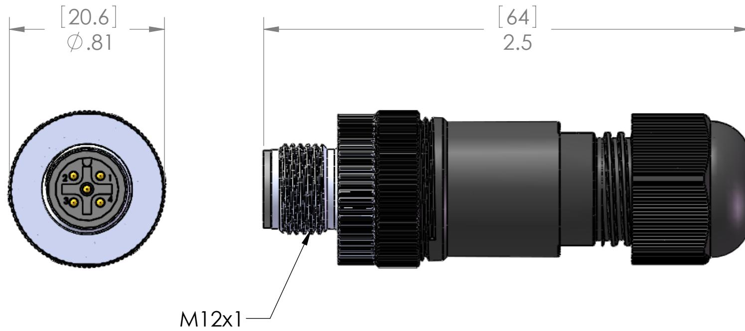
All connections made via Screw Terminals.
