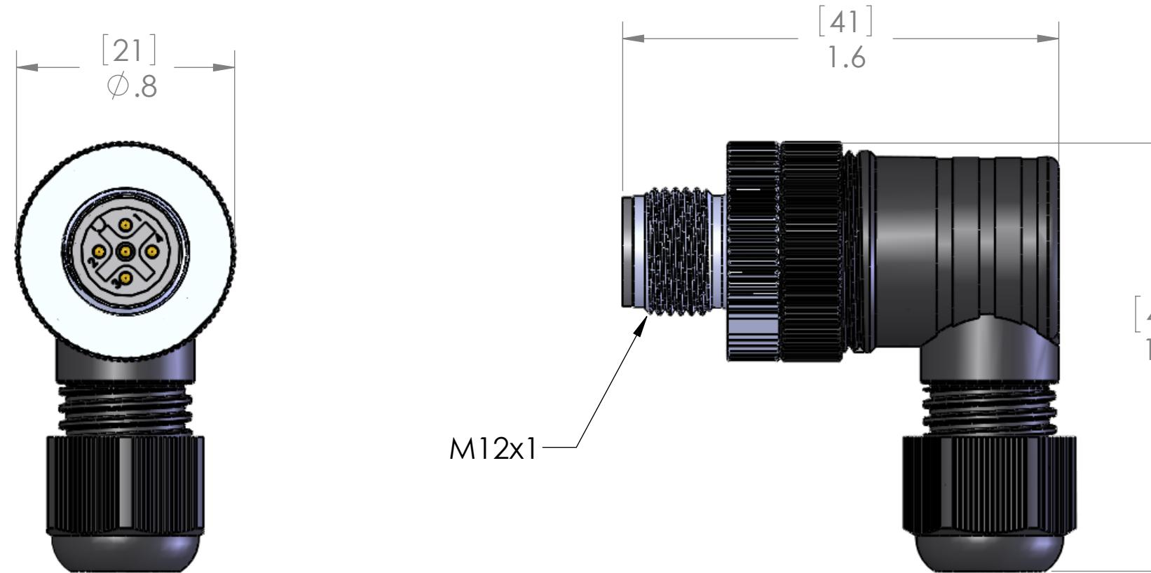
All connections made via Screw Terminals.
