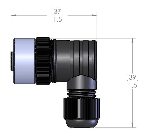
All connections made via Screw Terminals.
