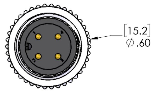
**PIN 1 CONNECTED TO PIN 2
