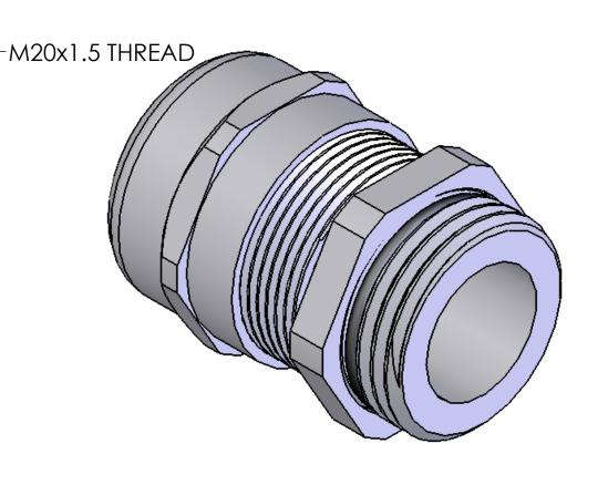
SEALING RANGE: 0.196" - 0.511" (5 - 13 MM) SEAL RATED TO: IP68 RECOMMENDED HOLE: 20.5MM
