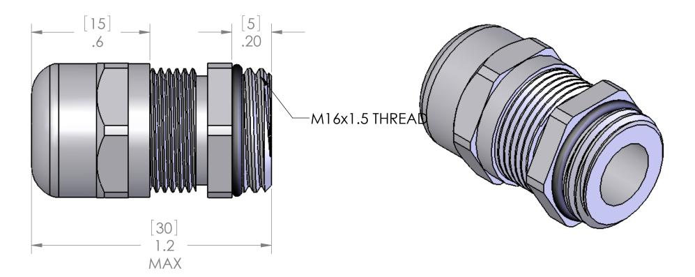
SEALING RANGE: 0.118" - 0.354" (3 - 9 MM) SEAL RATED TO: IP68 RECOMMENDED HOLE: 16.5 MM
