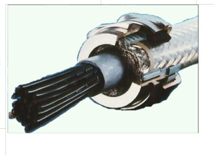
This is a shielding cable gland. For cables with a shield, the shield needs to be folded slightly around the gray plastic insert to allow the shield to be pinched between the gray plastic insert and the bottom of the gland.
