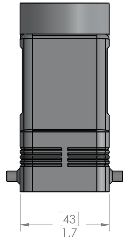
SEAL RATING OF IP 65 (IP66/IP69 WITH STAINLESS STEEL LEVER)
