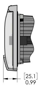
These devices shall be mounted on enclosures having adequate strength and thickness and with adequate spacing provided. Seal rating is based on mounting to a surface that is clean, flat and smooth.
