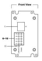
$1\sim5:10/100$  BASE-T(X) RJ45 ports  $6\sim10:10/100$  BASE-T(X) RJ45 LED  $11\sim13:$  Power Indication LED
