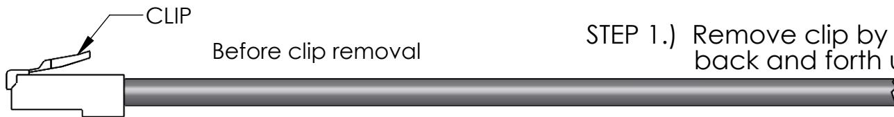
STEP 1.) Remove clip by cutting or by bending it back and forth until it breaks.
