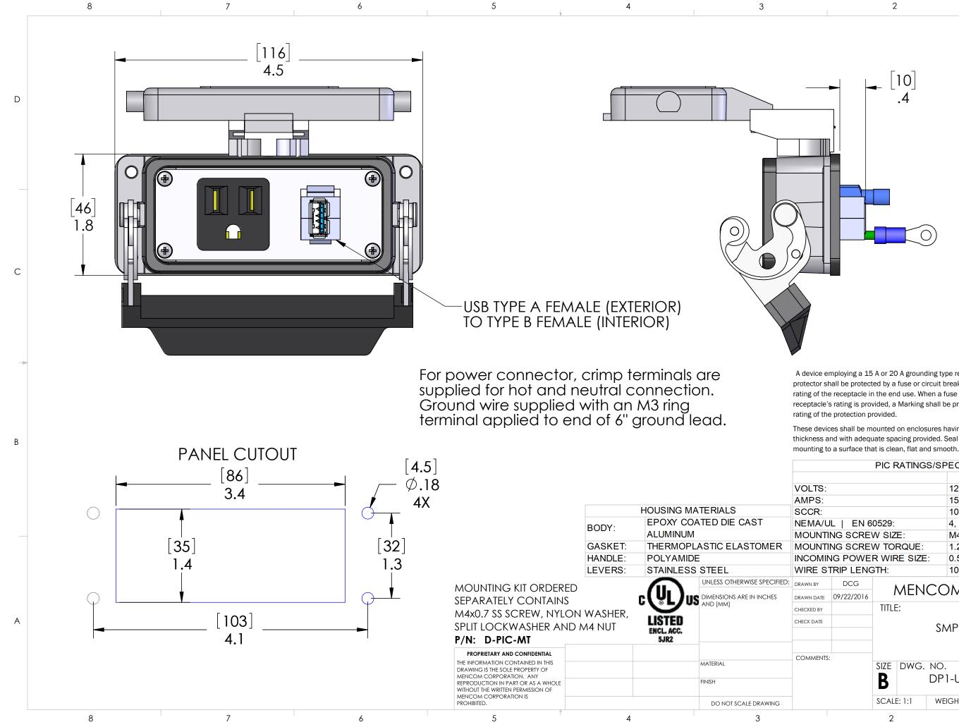
A device employing a 15 A or 20 A grounding type receptacle but no supplementary protector shall be protected by a fuse or circuit breaker that does not exceed the marked rating of the receptacle in the end use. When a fuse or circuit breaker rated less than the receptacle's rating is provided, a Marking shall be provided to indicate the maximum ampere
