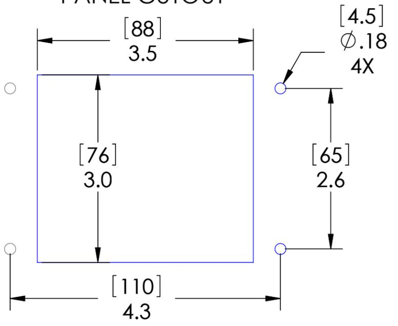
These devices shall be mounted on enclosures having adequate strength and thickness and with adequate spacing provided. Seal rating is based on mounting to a surface that is clean, flat and smooth.
