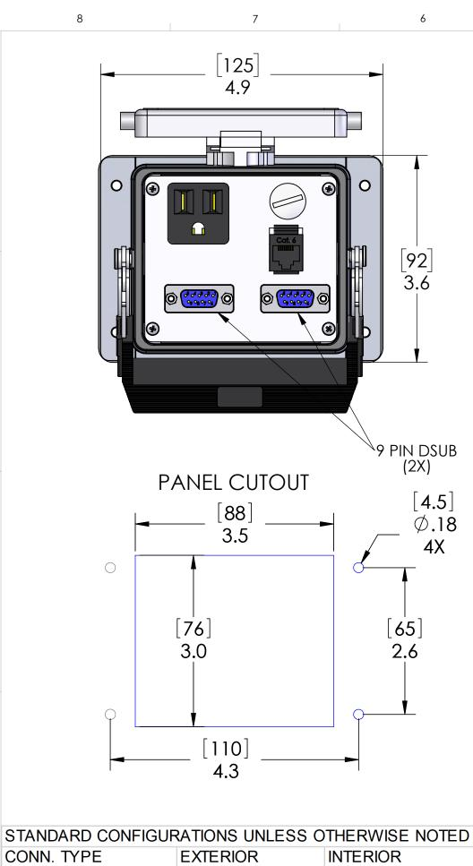
For power connector, crimp terminals are supplied for hot and neutral connection. Ground wire supplied with an M3 ring terminal applied to end of 6" ground lead.
