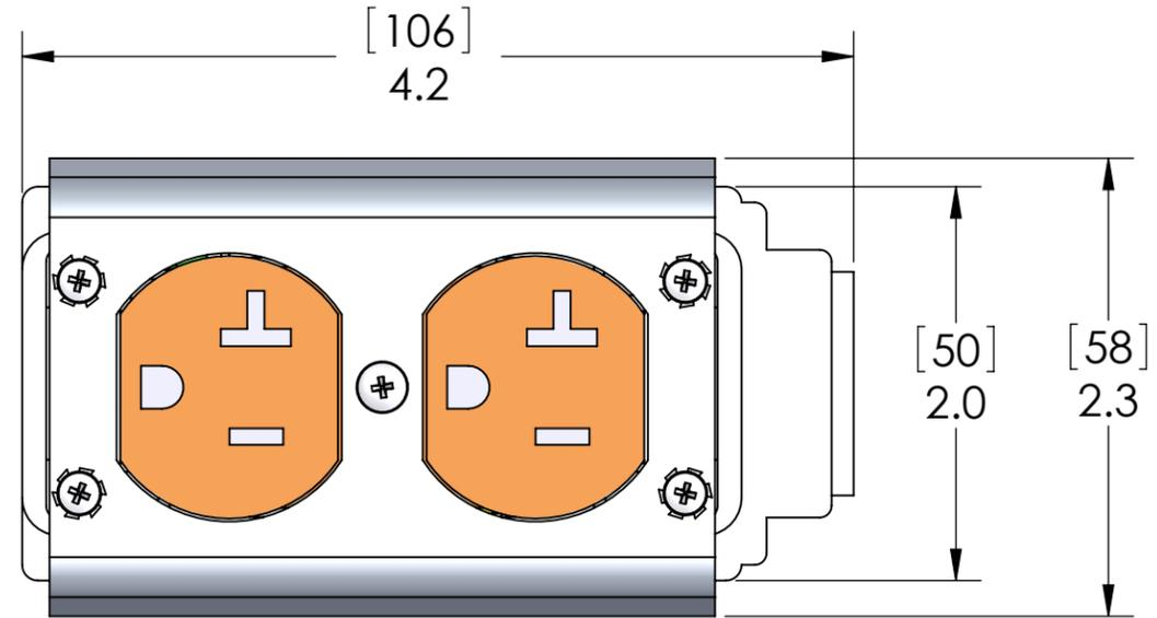
TS SYSTEM ALLOWS UNIT TO BE SNAP FASTENED ONTO DIN EN 50022 RAIL.
