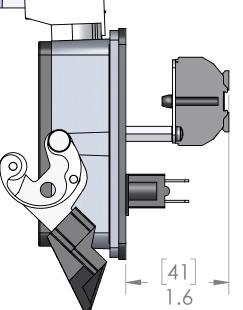
These devices shall be mounted on enclosures having adequate strength and thickness and with adequate spacing provided. Seal rating is based on mounting to a surface that is clean, flat and smooth.
