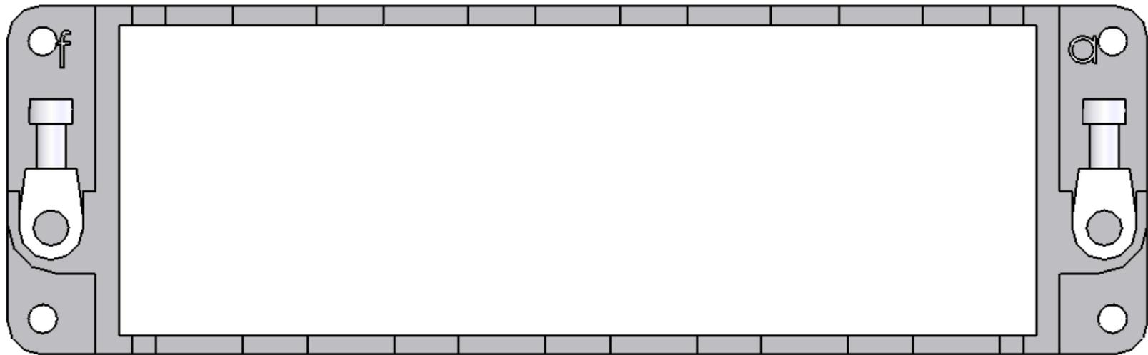
FRAMES CAN BE USED IN EITHER HOODS OR HOUSINGS, FOR CORRECT COUPLING PLEASE USE BOTH FRAME TYPES (ONE WITH UPPER-CASE LETTERS AND THE OTHER WITH LOWER-CASE LETTERS)
