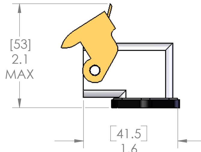
SEAL RATING OF IP 65 ONLY ACHIEVED WHEN FULLY LATCHED TO MATING BASE AND WITH AN APPROPRIATE SEALING GLAND INSTALLED AND WITH OPTIONAL CKR-65 SEALING KIT. OTHERWISE, IP44.
