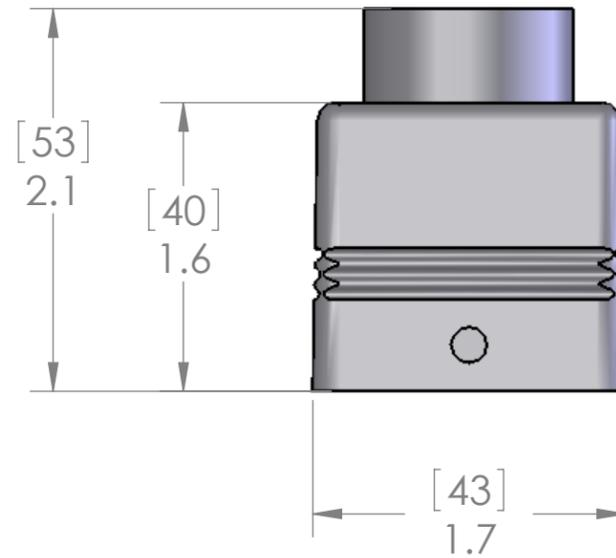
SEAL RATING OF IP 65 ONLY ACHIEVED WHEN FULLY LATCHED TO MATING BASE AND WITH AN APPROPRIATE SEALING GLAND INSTALLED
