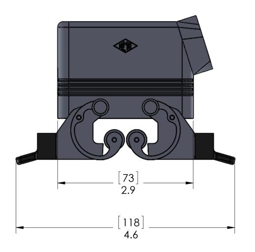
SEAL RATING OF IP 65 ONLY ACHIEVED WHEN FULLY LATCHED TO MATING BASE AND WITH AN APPROPRIATE SEALING GLAND INSTALLED
