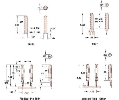
Alloy 260 Brass (70% Cu, 30% Zn. Higher Cu content resists dezincification Post-Ni = Brass, Nickel plated after stamping
