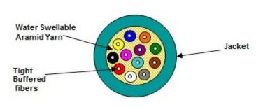
(Representation of a standard 12 fiber construction)
