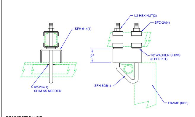
CONNECTION OF: FRAMEWORK ANGLE TO 2" CHANNEL FRAMING W/ 2" SPACER
