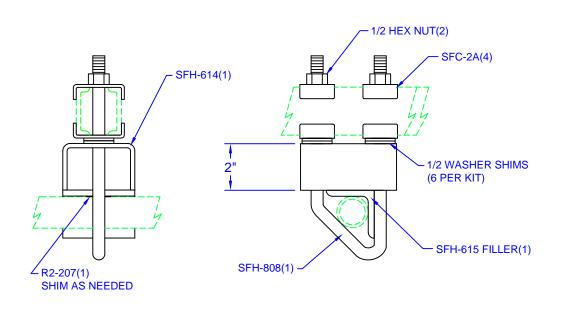
CONNECTION OF: SUPPORT PIPE TO 2" CHANNEL FRAMING W/ 2" SPACER (FUTURE FRAME LOCATION)
