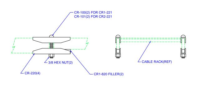
CABLE RACK SPLICE KITS(PR) 1-1/2" TO 2" SIDE BAR
