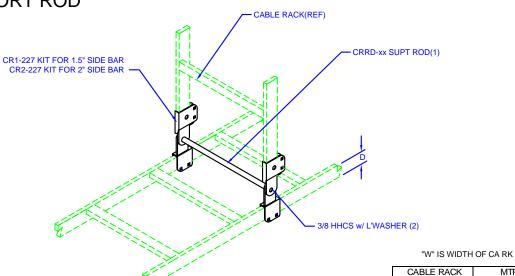
NOTE: FOR SPLICES WHERE CABLE RACKS HAVE DIFFERENT HEIGHT SIDE BARS: ORDER KIT FOR 2" SIDE BARS & (2) CR1-820 FILLER BARS
