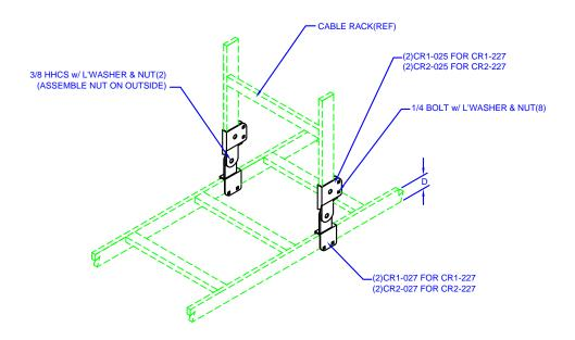
NOTE: FOR SPLICES WHERE CABLE RACKS HAVE DIFFERENT HEIGHT SIDE BARS: ORDER KIT FOR 2" SIDE BARS & (2) CR1-820 FILLER BARS
